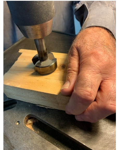
WRONG: Not using Clamps
