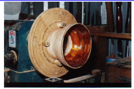
12 The top has been reversed on the Cole Jaws so that the inside could be sanded and given a coat of shellac.
