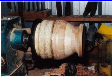
10 The rim at the top has been turned to the desired shape.
